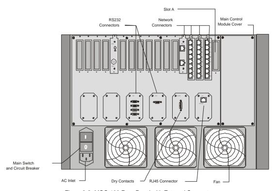
Figure 2-2: MGC-100 Rear Panel with External Connectors
